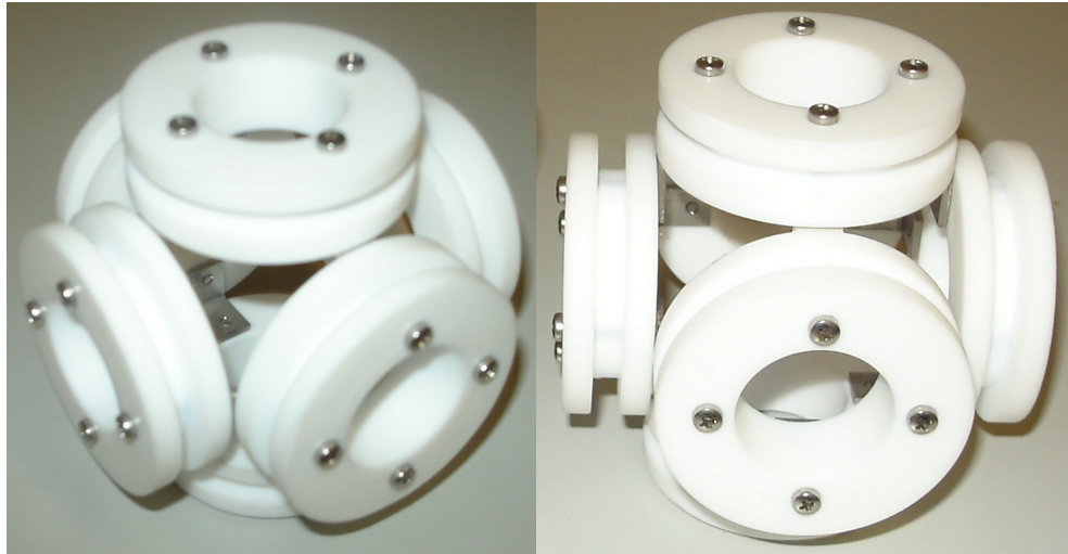
Figure 3.2: Two photos of the Teflon Polywell before adding coil windings. The left is orientated down the corner cusp revealing the aluminium angle bracket. The right image reveals the front view of the coil face.
