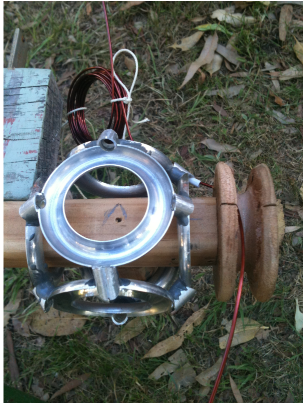
Figure 3.11: The inner toroidal shells are supported by a custom wooden jig used in coil assembly. The inner toroidal shells are joined with pre-cut pipe segments and JB-weld. On the end of the jig is a split-able coil former. One finished coil can be seen on the far side. A length of 15 m of wire was threaded through the joining pipe so that the next coil could be started. Once the coil winding was complete, the outer shells were clamped onto the frame with tensioned fencing wire.
