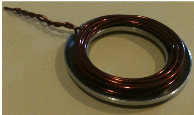
Figure 3.10: A single coil of 15 enamelled copper wire turns mounted into one of the finished half torus shells.
